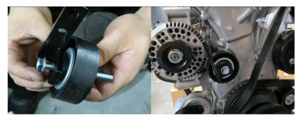
10. Take new 132277 bracket and install onto the engine front cover. Reuse top bolts and get hand tight.
