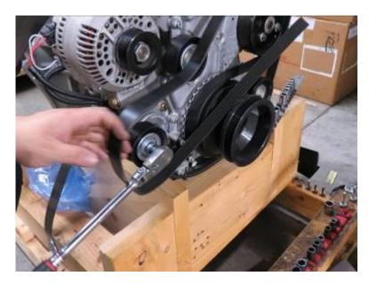
5. Using a 10mm socket, remove the idler pulley located next to the alternator
