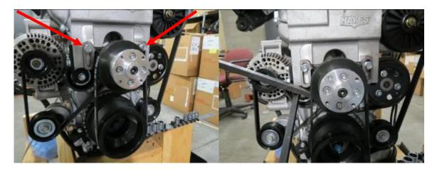
16. Use the original four bolts for the fan and reinstall the fan to the spacer. Torque 21 [ft-lbs].
