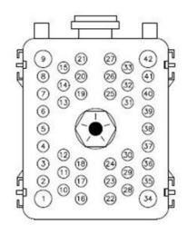
**Pin 1 (required) -** Connect to +12V switched ignition source. This pin must have 12 volts when the key is on. Remove voltage to shut off engine.
