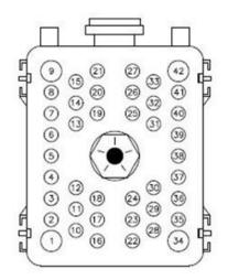
**Pin 1 (required)** – Connect to +12V switched ignition source. This pin must have 12 volts when the key is on.
