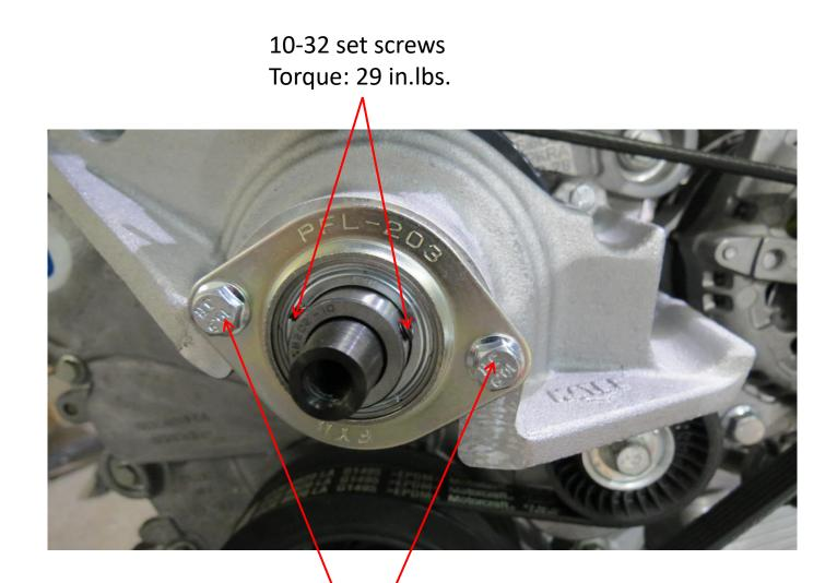
M6x1.0x16mm Bolts Torque: 71 in. lbs
