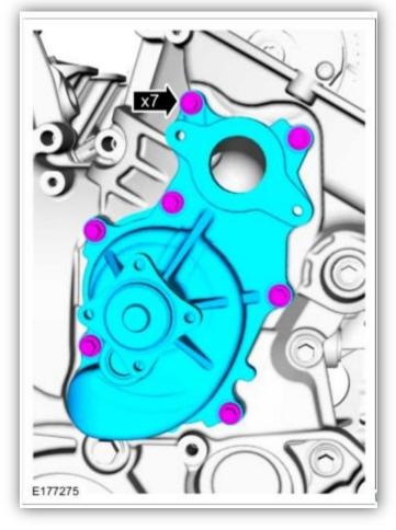
The front of the engine should now look like this, just a water pump remaining. We will now remove 3 bolts from the engine. 1- water pump bolt, 1-front cover bolt, and 1 thermostat housing bolt. These bolts can be discarded, they will not be needed for this kit. Tools required:
