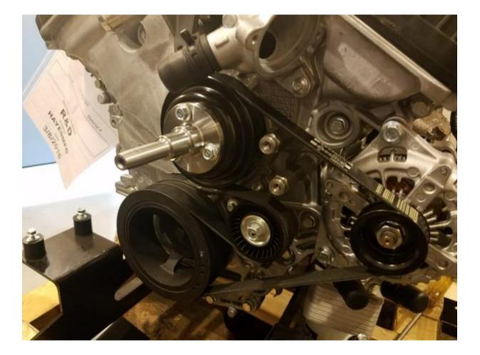
After assembling the fan support bracket we will install it on the engine.
