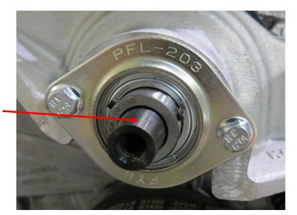
Install hub on taper Install 3/8-16X1" hex head, left hand thread bolt and 3/8" oversized washer Apply red Loctite Torque: 40 ft.lbs
