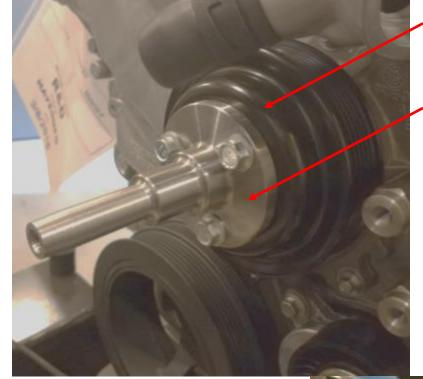
M8x1.25x20mm Flange head bolts Torque: 26 ft.lbs.
